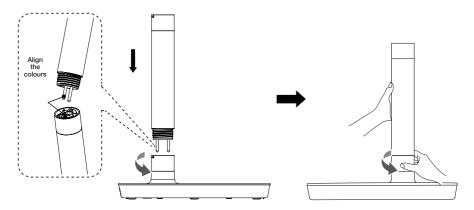
To attach the column/s and air circulator head align the gold metal guide pin with the gold hole and insert to bring the poles together. Turn the security collar counter clockwise until it is securely tightened.
