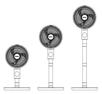
Assemble the air circulator according to your preference. The column/s can be attached for increased height or the air circulator head can be attached directly to the base creating a table air circulator.
