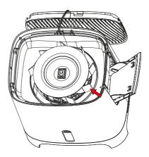
(5) Repeat the above process in reverse to put the humidifier back together.
