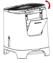
The grill will stay connected to the humidifier, rest it on the side.
